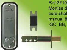
Mortise dead bolt (25mm throw) hardened steel core shaft for additional security, 60mm back set, manual throw back to re-lock -SC, BB, AB, AC & JB finishes
